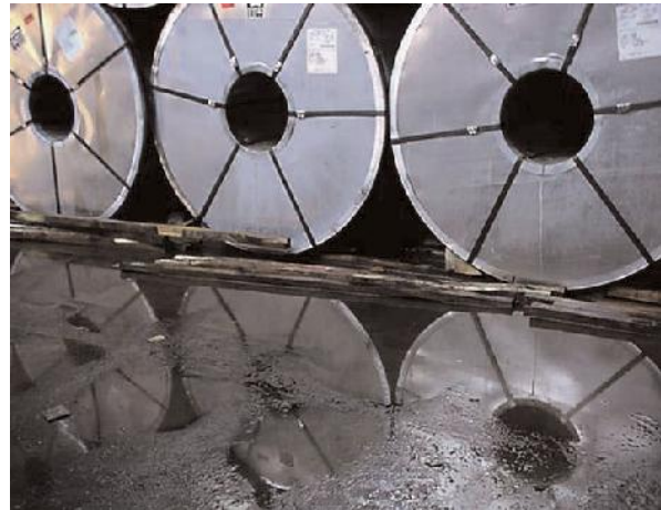
Photo 2. Coils of cold rolled steel The higher quality surface finish of cold rolled steel makes it much more susceptible to rust damage. It is for this reason that cold rolled steel is usually packed in bituminous paper and kept away from moisture
