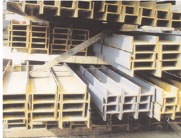
Photo 4. Constructional steel ('1' beams) Note that the beams are stacked correctly, with the flanges 'in and out'
